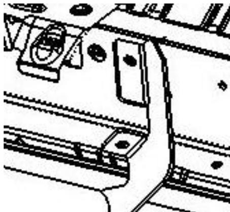
**Step 4** After final adjustment tighten all the lower mount first then the upper mounts.
